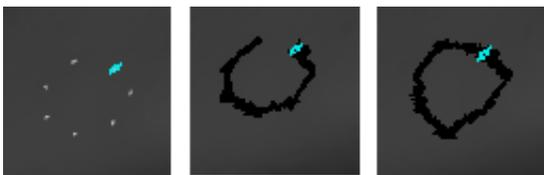
The Cut Plane tool requires exactly four marked vertices. The first three define three points on the plane and the fourth defines a point inside the plane. This image shows this process. The surface image has been scaled down to show that the entire surface has been cut away in the second image.
